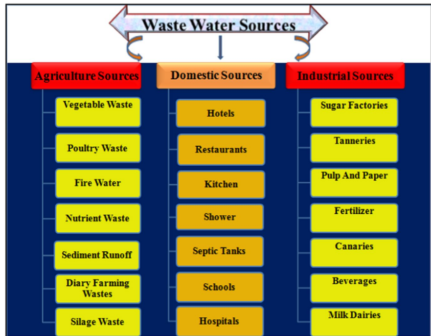
Fig. 1 Schematic representation of various wastewater sources
