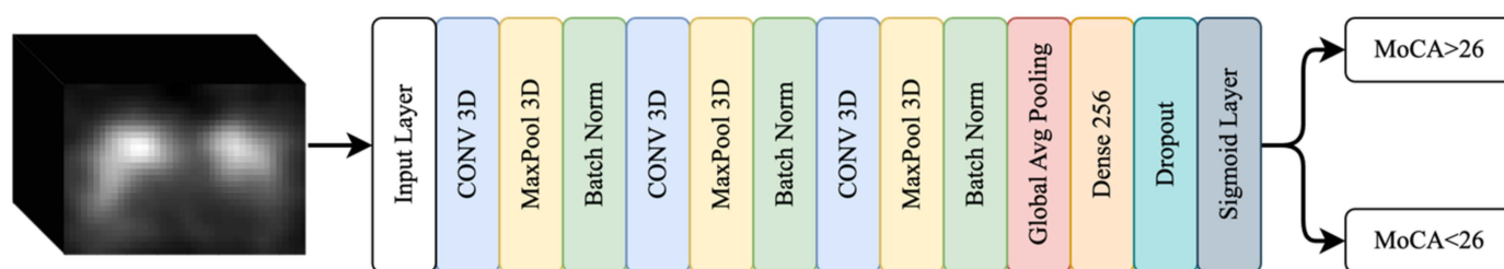
Figure 4. A schematic diagram of the proposed convolutional neural network consisting of 13 layers including three 3D convolutional (CONV) layers, three max-pooling (MAXPOOL) layers, and three batch normalization (BN) layers passed to a fully connected layer with 256 neurons.
