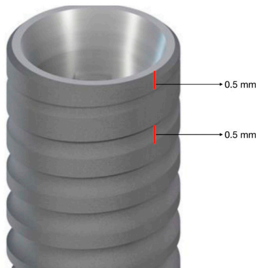
Figure 9. Schematic representation of the implants used in the study with indications of the distance between the platform and the first thread, as well as the distance between the threads.
