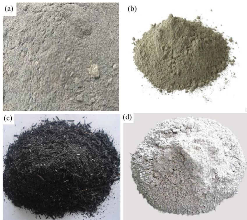
**Figure 4.** The main forms of aluminosilicate raw materials used in the technology of geopolymer concretes (a) fly ash, (b) metakaolin, (c) rice husk ash, (d) ground granulated blast furnace slag.
