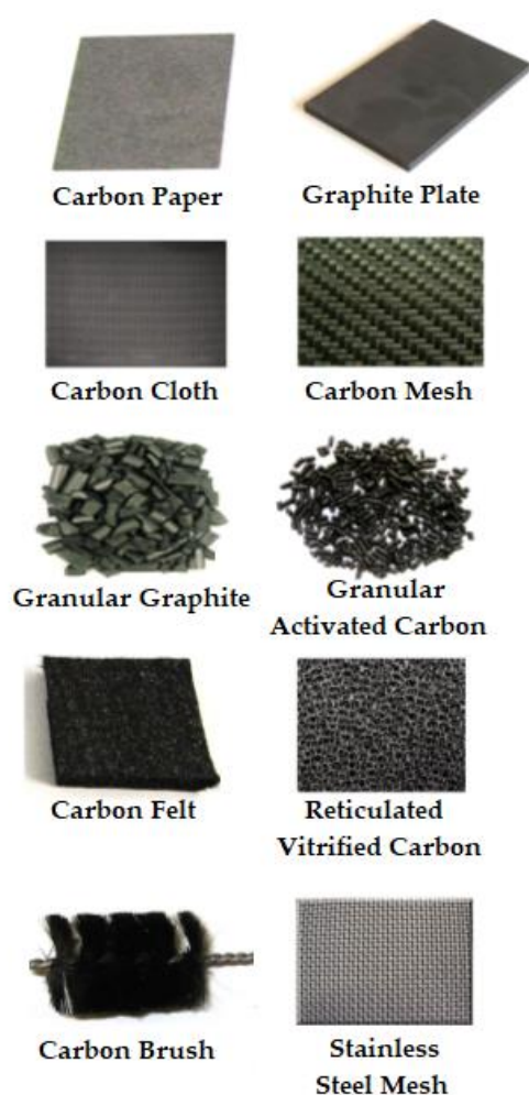
Figure 2. Different anode materials used for microbial fuel cells [adapted and modified from reference [22] with permission, 2023, Elsevier.
