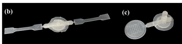
Figure 1. The schematic diagram for preparation of the PLLA/PPDO blend microparts (a), the digital picture of the micro tesile sample (b) and the microneedle array (c).
