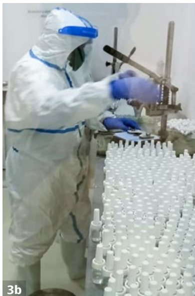
Figure 3 a. Amber glass bottles with PPE plastic droppers. b. Manual capping/sealing of bottles. c. Visual inspection area.
