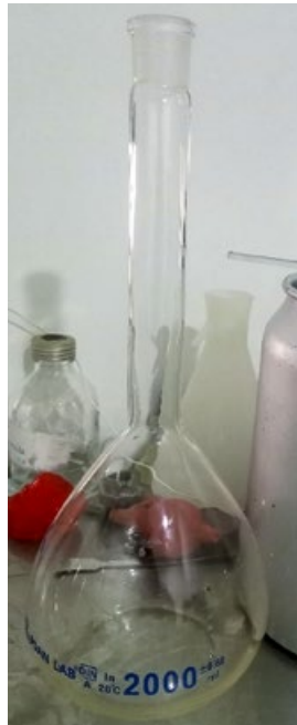
Figure 2 Volumetric flask (2,000 ml) for dilution of chlorhexidine 20% w/v to 0.2% w/v by addition of acetate buffer.
