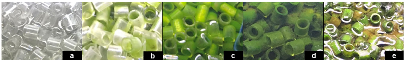
Fig. 2 Biofilm development with microalgal-bacterial consortia on carrier media. a 0 h, b 380 h, c 550 h, d 720 h, e 1200 h
