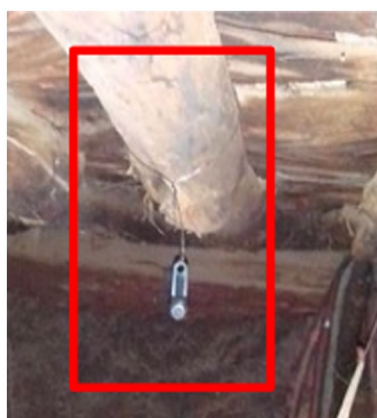
FIGURE 4 Installed sensor that measures indoor temperature and humidity, which is part of the household-level data collection in CHEERS.
