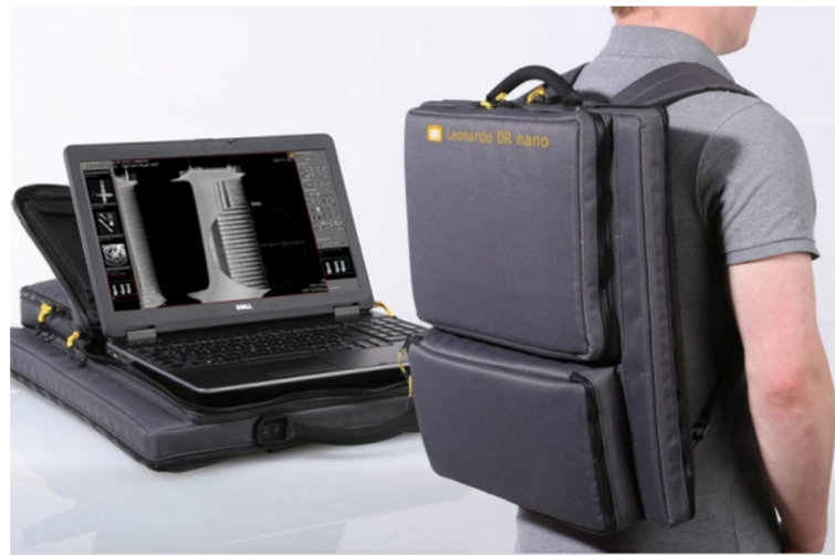
Figure 1. Image of a Leonardo nano mobile X-ray system.
