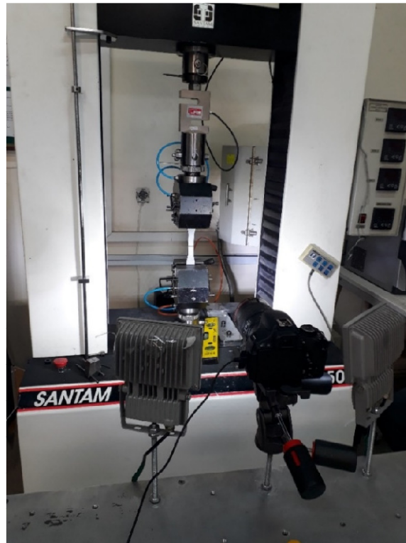
Figure 7. Experimental setup for the tensile tests, including the DIC equipment.
