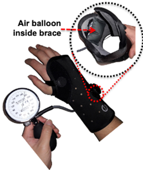
Fig. 7 Wearable brace with inflatable balloon bladder in the brace for radio ulnar wrist compression
