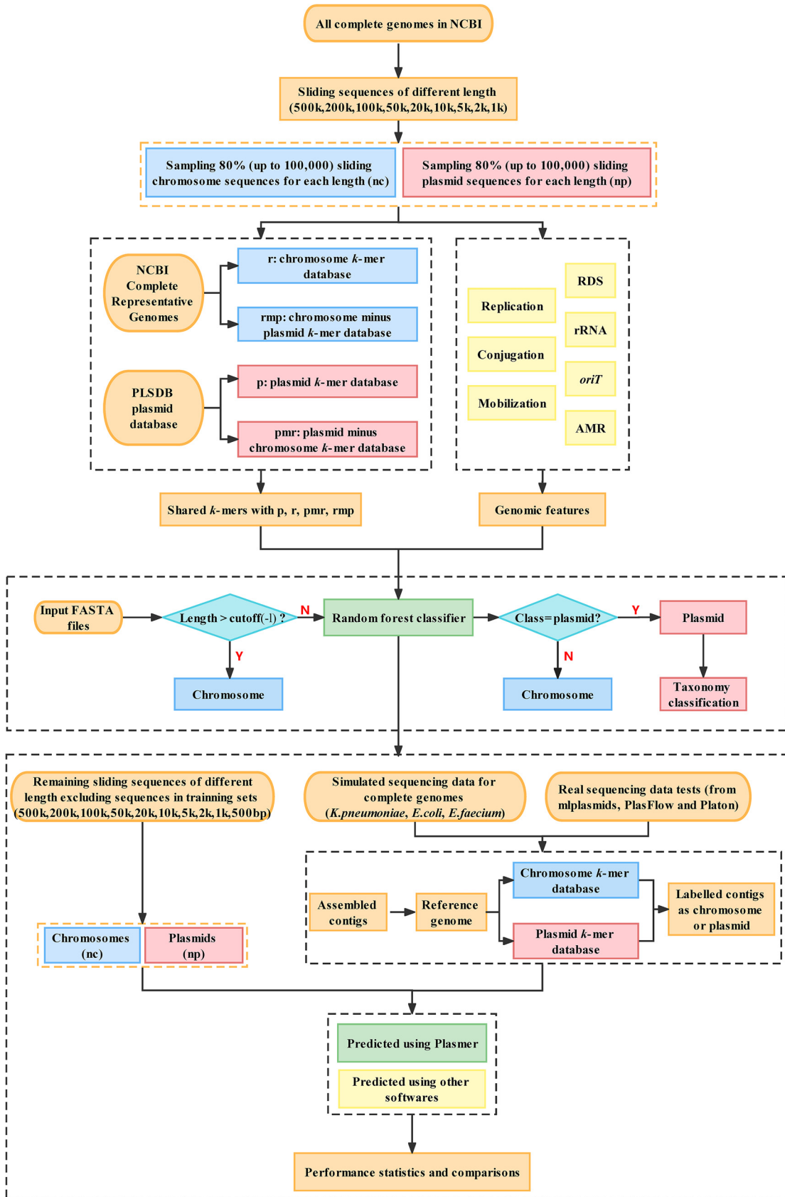
FIG 5 The workflow of Plasmer. The nc and np boxes represent the chromosomes and plasmids, respectively, of 31,897 complete bacterial genomes in NCBI. The r, p, pmr, and rmp boxes represent the k-mer database from chromosomes of
