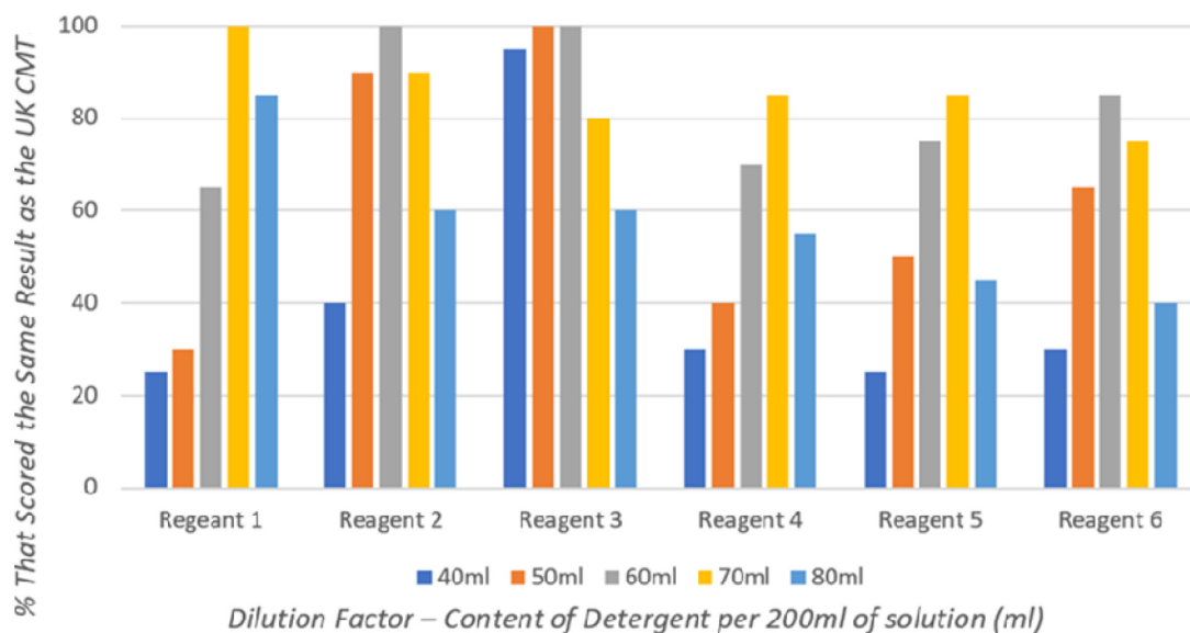
Figure 1. The percentage of detergent-based CMT results that achieved the same result as the commercial UK CMT for each different dilution when testing 20 milk samples.
