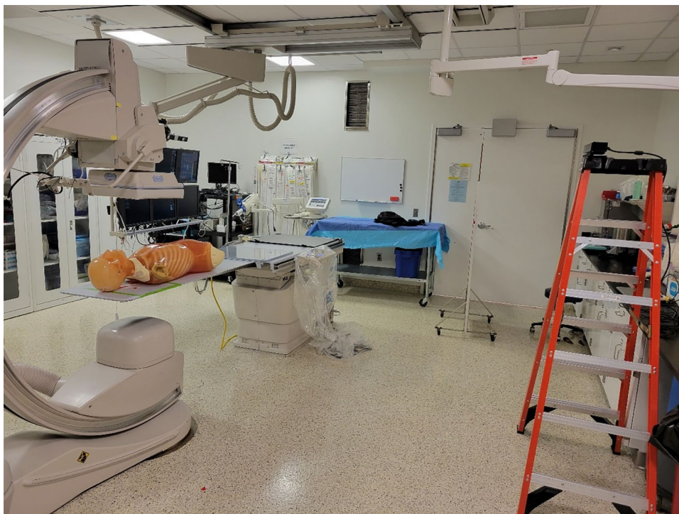
Fig. 8 The set-up used for the simulated procedure. A Kyoto-Kagaku anthropomorphic phantom was placed on the catheterization table to simulate a cardiac interventional procedure. The Kinect V2 camera is shown to the right in this image, and is fixed to the top of the ladder. This camera was used to record the procedure, as well as the coordinates of one individual's waist
