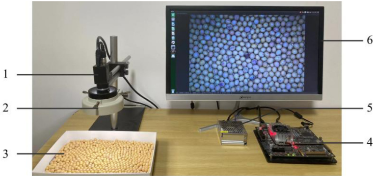
Note: 1. industrial camera; 2. light source; 3. soybean seeds; 4. NVIDIA Jetson TX2; 5. power supply; 6. display.
