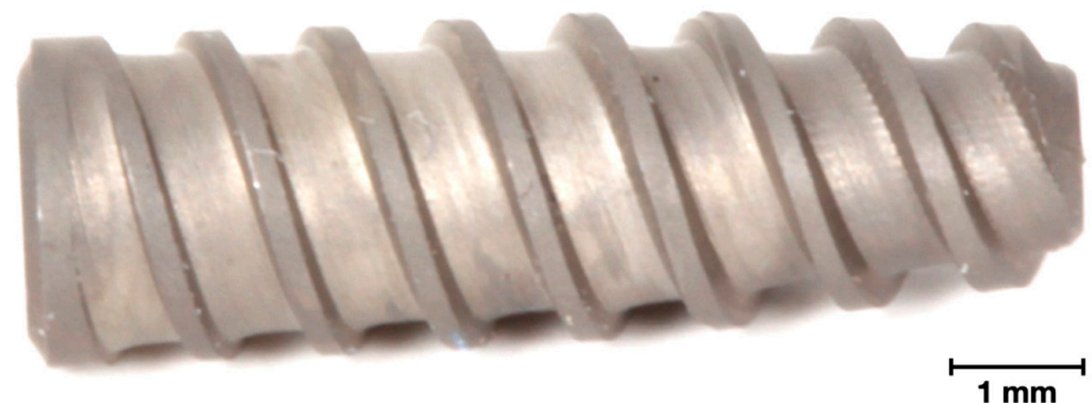
Figure 1. Figure depicting the design of the conical screw-type acid-etched type V Titanium alloy implant used in the current study.
