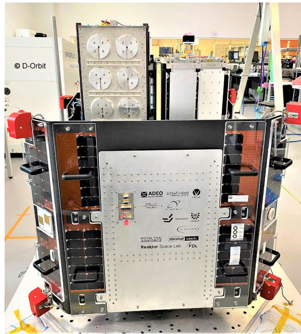
Figure 1. Picture of the D-Orbit ION Satellite Carrier Dauntless David being prepared for launch. After reaching LEO on board a SpaceX Falcon 9 rocket the satellite disconnects and ferries client SmallSats into custom orbits. The satellite also carries internal hardware payloads, one of which is D-Orbit's Cloud Computing in Space module, which is used to run the WorldFloods ML payload. Image used with permission of D-Orbit.
