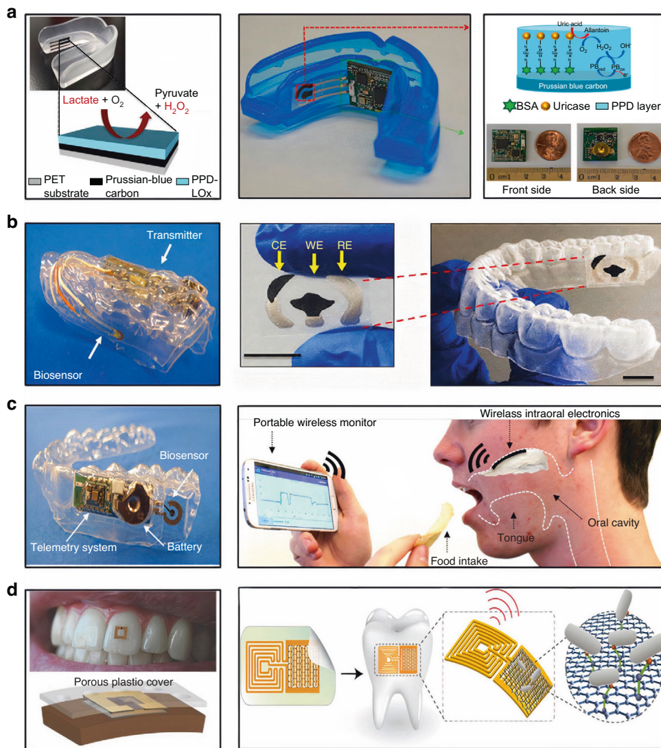
Fig. 4 Summary of wearable intraoral biosensing platforms for non-invasive salivary analysis. Lactate biosensor on a mouthguard ( a , on the left). Reproduced with permission from Kim et al. 86 Mouthguard with biosensor and integrated electronics for real-time uric acid detection ( a , on the right). Reproduced with permission from Kim et al. 86 Mouthguard with screen printed electrodes for N-Carboxymethyl lysine detection ( b ). Reproduced with permission from Ciui et al. 177 Glucose biosensing telemetry system ( c , on the left), reproduced with permission from Arakawa et al. 178 and a hybrid flexible bioelectronic platform for sodium monitoring ( c , on the right). Tooth mounted hydrogel radiofrequency biosensor ( d , on the left), reproduced with permission from Tseng et al. 179 and graphene-based biosensor for pathogen's detection ( d , on the right), reproduced with permission from Mannoor et al. 99
