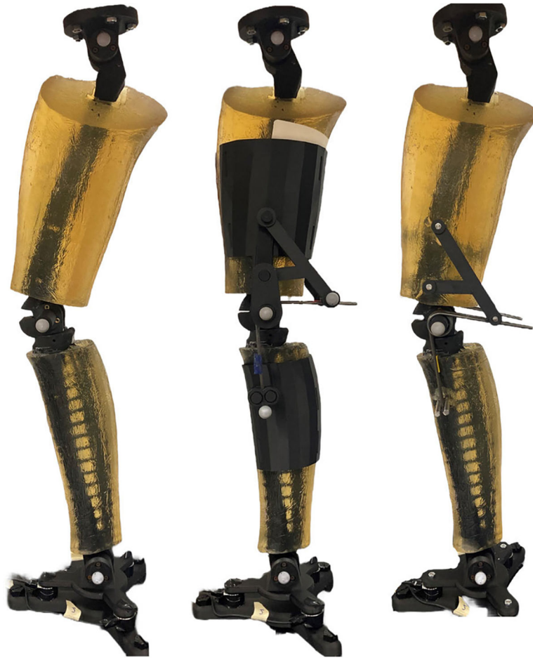
Fig. 4. The phantom lower limb mounted on the hexapod under various loading conditions. The left image presents the phantom without any springs or braces. Middle image shows the phantom with torsional springs attached to braces interfacing the ballistic gel of the thigh and shank. The right image shows the phantom with the same springs bypassing the ballistic gel and attaching directly to the femur and tibia. Load cells attached under the ankle and marker positions at the joints are used to estimate the knee moment.
