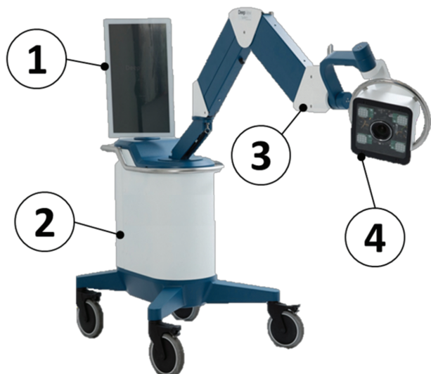
Figure 1. The multispectral imaging device utilized for this study. The system include: (1) a touch-screen display; (2) mobile cart containing the processing unit; (3) an articulating arm to position the camera; and (4) the MSI subsystem. MSI, multispectral imaging.
