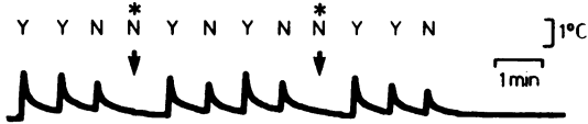
Fig 2 Example of the sequence of thermal stimuli and subject's responses during a test. "Catch trials" are marked with an asterisk. To prepare this figure the output from the thermocouple in the thermode was connected to a chart recorder.
