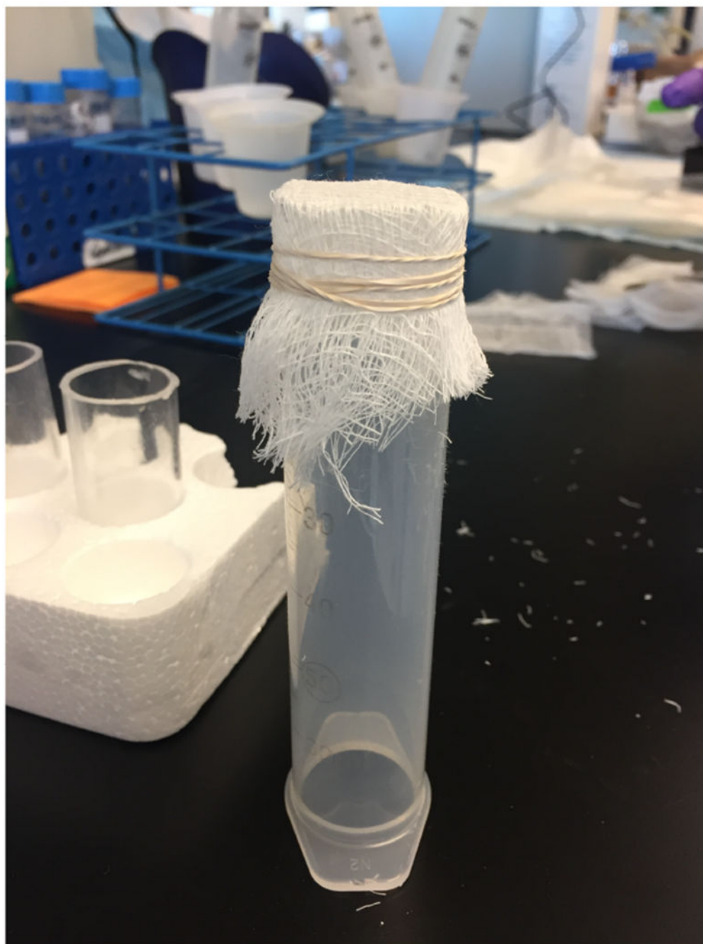
Fig. 5. Filtering device made from a 60 ml syringe with the needle adaptor cut off. The filter, made of layered gauze, is attached using a rubber band.
