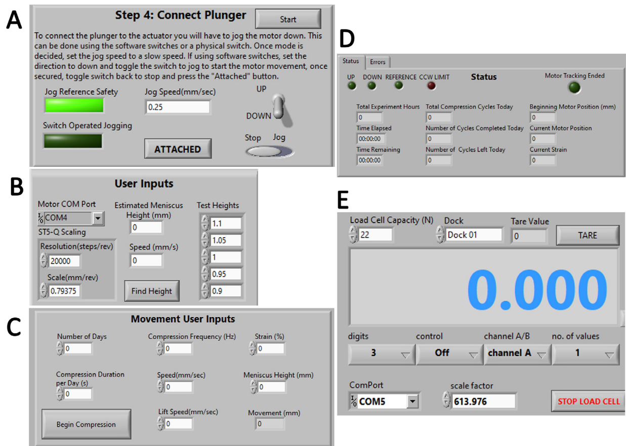
Fig. 6. Operating Software Graphical User Interface Panels. (A) A hardware configuration panel provides instructions for actuator control; (B) Height measurement program panel allows probing of multiple test heights; (C) Strain-based compression program allows for long-duration compression cycling; (D) Compression cycling status display; (E) Load cell reading and tare panel.
