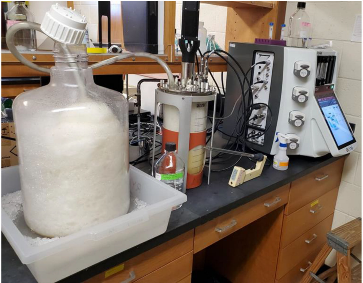
Figure 1. Bioreactor-dependent apoE4-NT-induced foam production. Photograph obtained 5 h post-induction of apoE4-NT expression depicting the bioreactor control panel (right), culture chamber (middle) and foam collection vessel (left). As foam fills the bioreactor chamber, it is forced out through flexible tubing attached to a headplate port and into a 30 L carboy collection vessel. The foam deposited in the carboy is dense and piles up on itself to occupy a large volume of the collection vessel.
