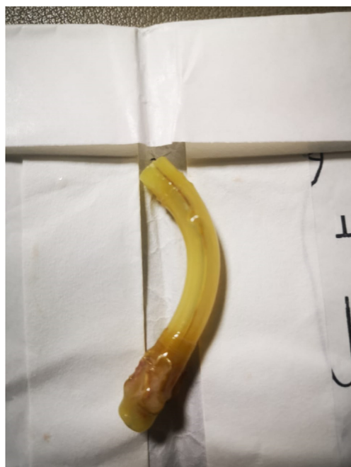
Fig. 3 – Fractured tracheostomy tube after removal.
