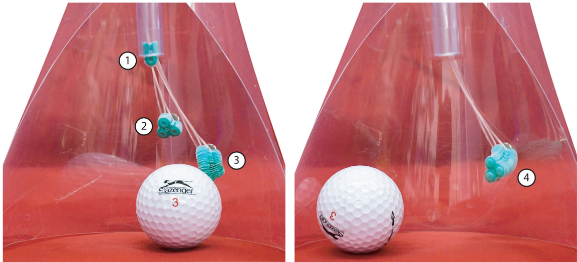
Figure 10: Demonstration of squeezing through a small aperture and operating in a large workspace. The 3-DoF SBA begins folded inside a lumen of diameter d = 9.25 \text{ mm} (1). It then exits the lumen and is fixed to a wall via an external magnet (2). From its fixed position, it expands to move a golf ball (3–4).
