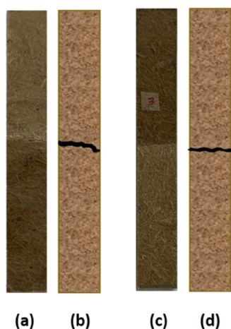
Figure 5. Composite sample failures after the flexural test: (a and b) UT composite real failure and illustrated failure, respectively; (c and d) AT composite real failure and illustrated failure, respectively.
