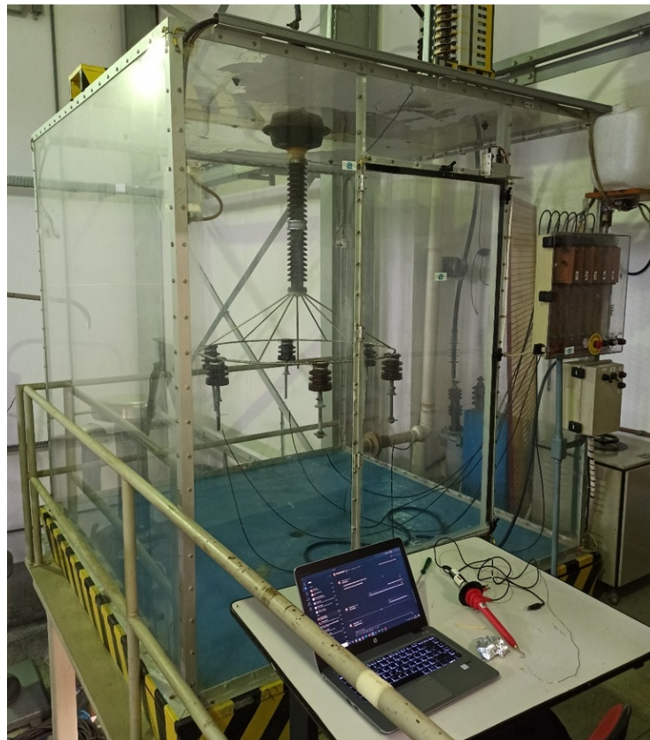
Figure 1. Salt fog chamber (high-voltage laboratory).
