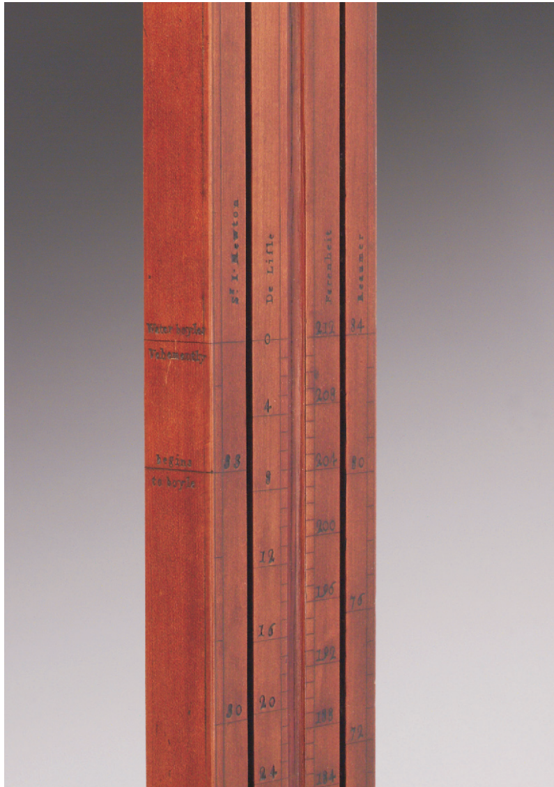
Fig. 1. George Adams's thermometric scale, showing two boiling points (inventory no. 1927–1745). Science Museum/Science & Society Picture Library.
