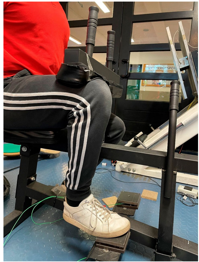
Fig. 3 Calf muscle testing device equipped with force plates to measure maximal isometric strength with flexed knee joint (MVC90)
