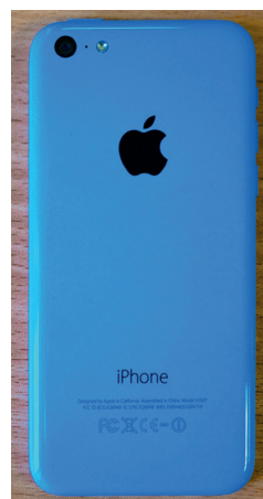
Figure 4 Smartphone with a polycarbonate unibody shell. Credit: Kārlis Dambrāns, https://upload.wikimedia.org/wikipedia/commons/a/a6/IPhone_5c_blue_back.jpg .
