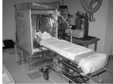
Figure 6 Experimental arrangement for measuring oxygen concentrations in human subjects at the Dartmouth Medical School with a 50 cm sample cavity. Note vast difference in size from the set-up in Figure 5. Reproduced with permission. http://www.dartmouth.edu/~eprctr/research/tooth_dosimetry.shtml
