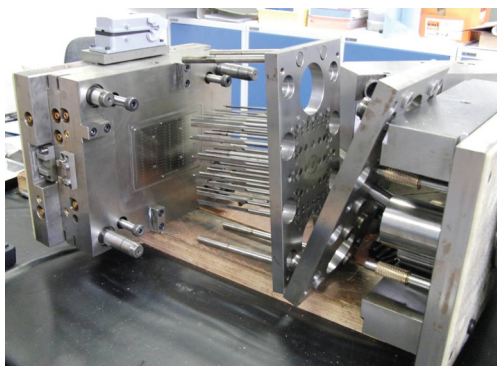
Figure 6 Injection moulding tool for microfluidic devices with the size of a microtiter plate. Note the mechanical complexity.
