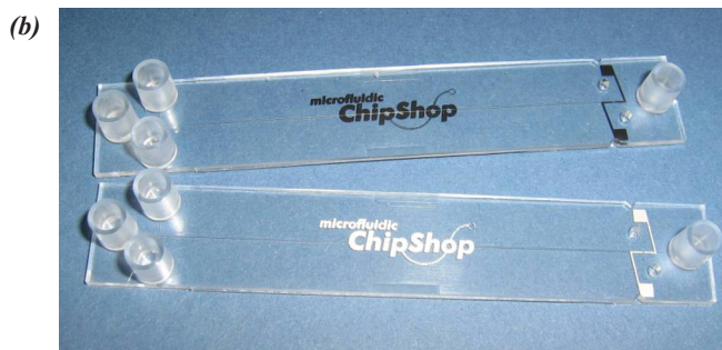
Figure 16 Instrument for chip-based capillary electrophoresis (a) and associated microfluidic chip (b).
