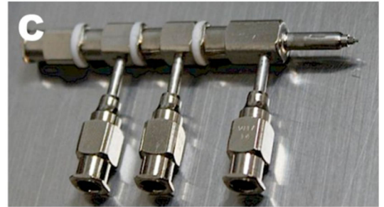
Fig. 1. (A) Co-axial ES apparatus for generation of acetalated dextran (Ac-DEX) microparticles encapsulating the adjuvant resiquimod and a protein antigen in a single microparticle [11]. (B) Co-axial needle [12] and (C) Tetra-axial needle [12]. The Taylor cone would be created at the right-hand tip, with Luer-Lock style imports at the left and facing down.
