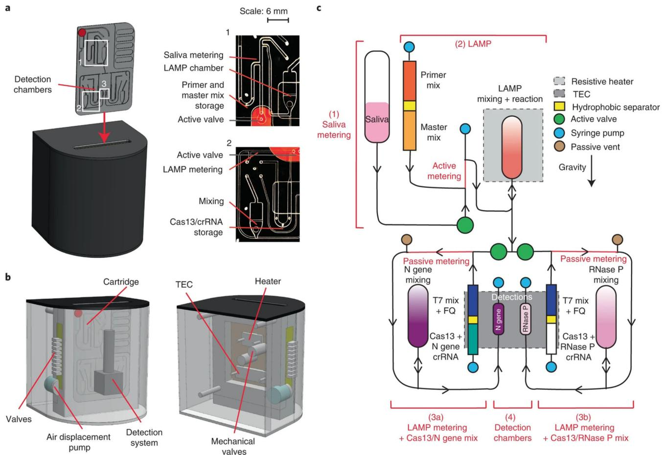
**Fig. 6 | Design of an automated microfluidic-driven diagnostic system.**
