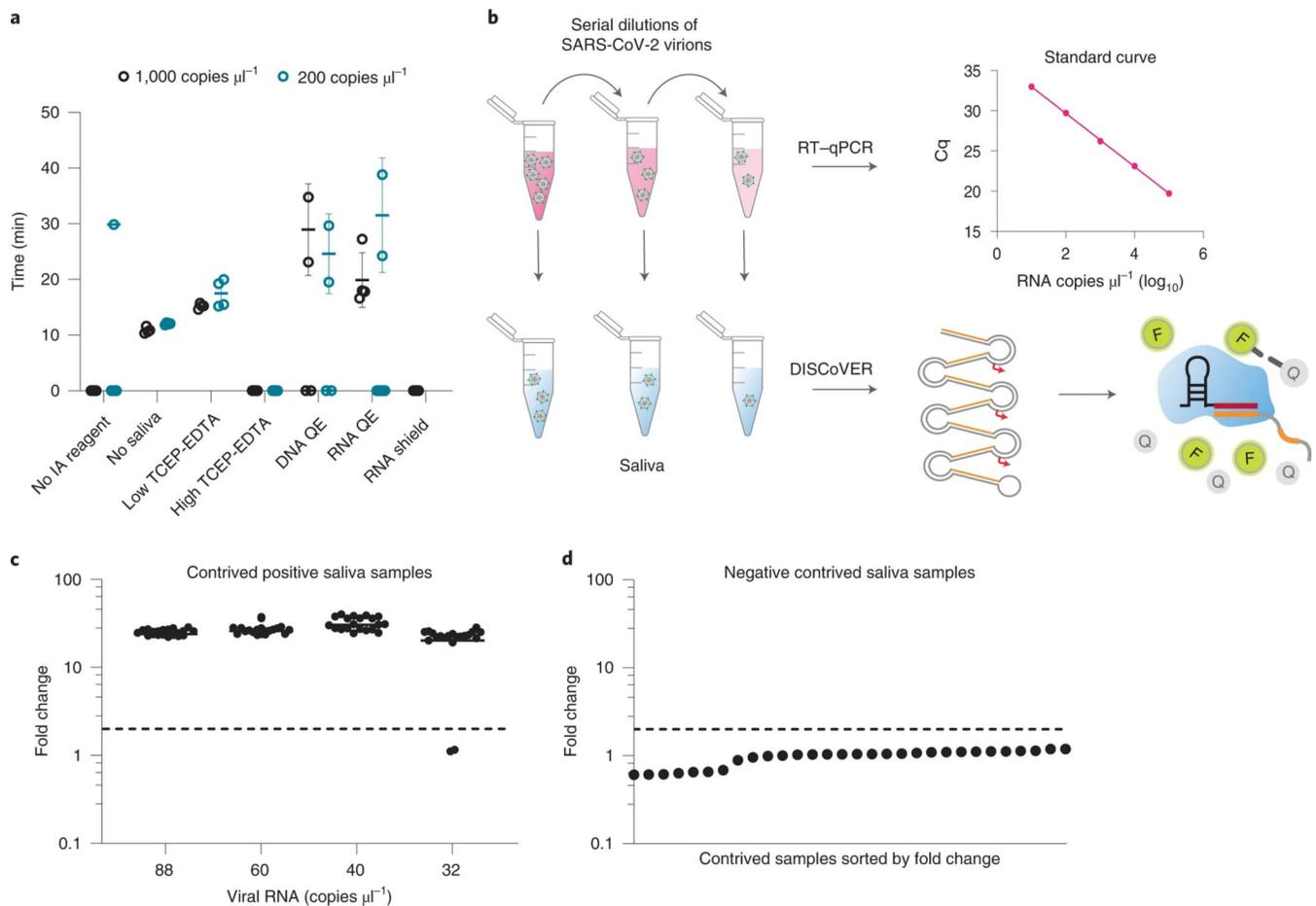
**Fig. 4 | DISCoVER for extraction-free detection of saliva.**
