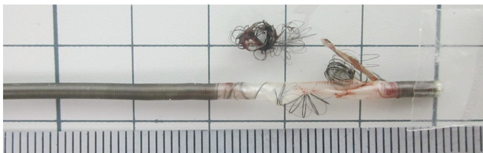
Fig. 5 Damaged JET 7 Xtra Flex. The JET 7 Xtra Flex was broken at a site 5 mm from the tip by 25 mm toward the proximal side, the outer layer polymer was torn in a 20-mm range, and the coil wind was fully stretched and popped out.
