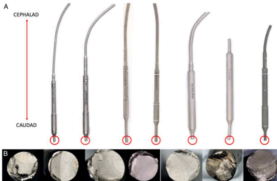
Fig. 4. Showing (a) macroscopic images of 7 single construct MAGEC X rods that fractured in situ and (b) the fracture sites of each rod with features characteristic of fatigue fracture (Tognini et al., 2023).
