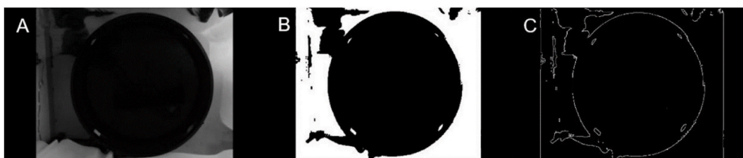
Fig. 2. Process followed to obtain the contour of the pool. (A) Projection of minimum intensity of the pixels through the stack. (B) Binary image. (C) Contour of the pool, obtained by mathematical morphology.
