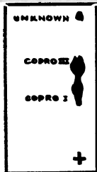
FIG. 5.—Chromatogram of porphyrin methyl esters prepared from urine in lead poisoning. Photograph of spots red-fluorescent in ultra-violet light. Solvent oleic acid-kerosene (1 : 1).
