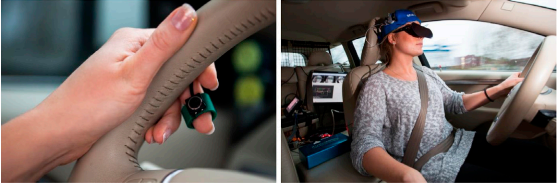
Figure 2. An example of a visual occlusion mechanism that is activated by a micro-switch placed on the middle finger from the on-road study by Kircher et al. (2020).
