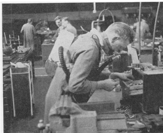
FIG. 2.—Tool-room operative fitted with respirometer for measuring and sampling his expired air during work. A globe thermometer and other instruments used for assessing environmental warmth are shown on the trolley behind the subject.
