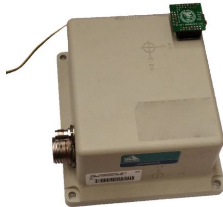
Figure 7. MEMS sensor array mounted at the top of the FOG unit.
