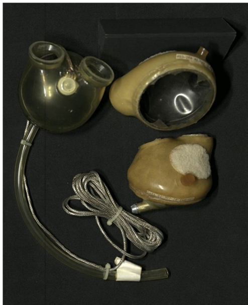
Fig. 2 Kolff and Atsuku total artificial heart. Reprinted with permission. https://blog.lib.utah.edu/father-artificial-organs-willem-j-kolff/
