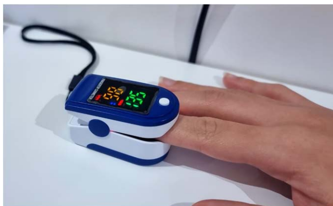
Figure 2. A pulse oximeter device for the non-invasive measurement of arterial oxygen saturation, available from pharmacies for home monitoring.
