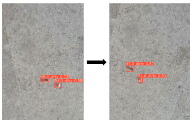
Figure 8. Tracked detections in sequential frames using real-time video footage. Here, the class 'dirty' on the bounding boxes refers to solid dirt.
