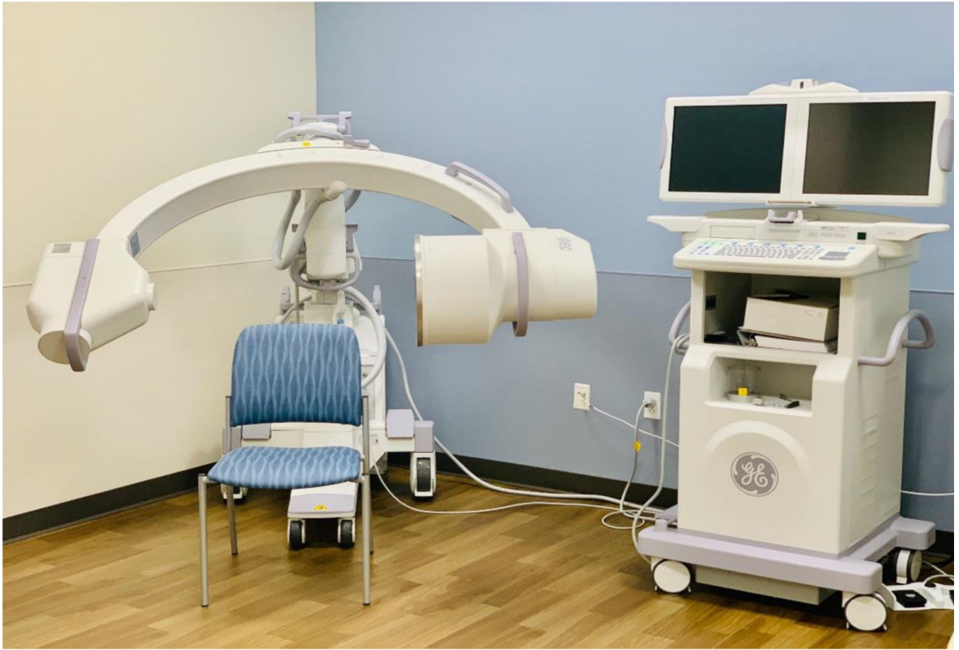
Figure 2. Mobile C-Arm Fluoroscopy machine. The patient sits in a chair while a VFSS is conducted to evaluate oropharyngeal dysphagia.
