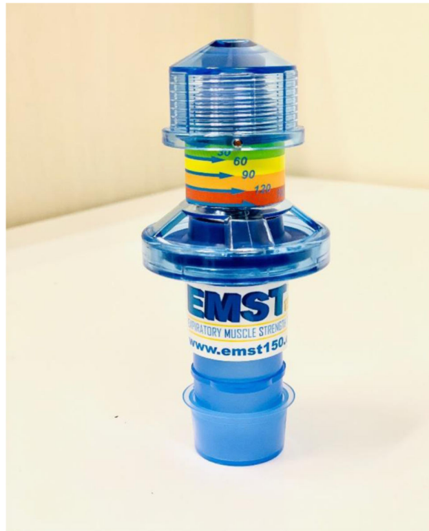
Figure 5. Example of an expiratory muscle strength training device. Image of the EMST 150 ® pressure-threshold device; (Aspire, LLC; Atlanta, GA) used as a rehabilitative strategy to strengthen expiratory muscles. The device consists of a calibrated, one-way, spring-loaded valve and pressure resistance can be set from 30–150 cmH 2 O.
