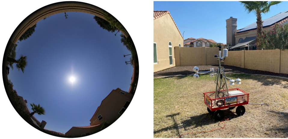
Figure 3. The MaRtY human-biometeorological station located in a single-family home backyard in an open low-rise Local Climate Zone (LCZ 6, SVF: 0.909) neighborhood in Phoenix, Arizona. The portable station monitors net radiation in three directions to provide highly accurate MRT values, air temperature, relative humidity, and wind velocity.
