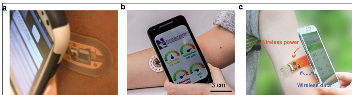
Figure 25. Wireless energy harvesting from the mobile phone.
