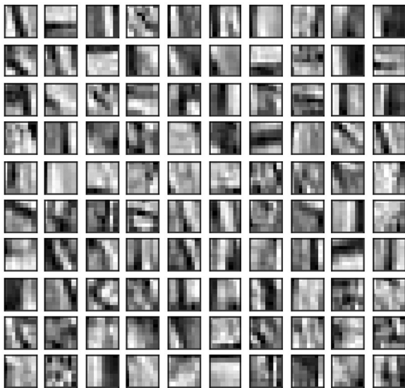
Fig. 1 Representative display of an overcomplete dictionary from noisy patches. A matrix of vectors with more representative columns than rows is created using a modified least angle regression algorithm (LARS) which serves as an individualized “noise map” for the subsequent Orthogonal Matching Pursuit (OMP) denoising algorithm
